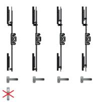
Only with the anti-false manuever mechanism engaged, it will be possible to proceed with the system's locking, ensuring a smooth and ideal closure while significantly reducing the possibility of damaging the locking points or multipoint lock mushrooms.
